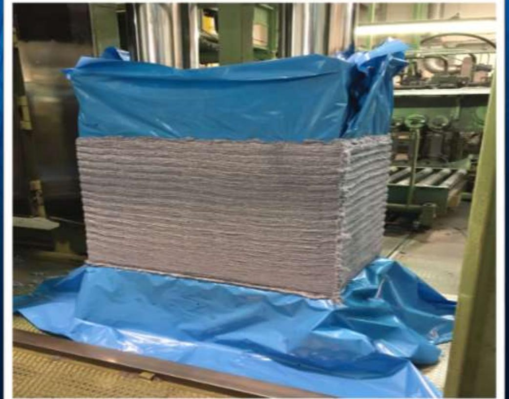
AND PACKED IN BALES TO BE SENT INTO THE SPINNING PROCESS
